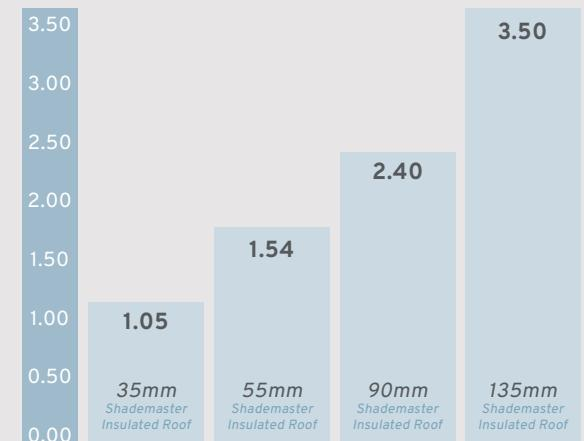
All calculations for the above are based on a mean temperature of 23°C in compliance with AS 4859.1:2002 Section 2.3.3.3
